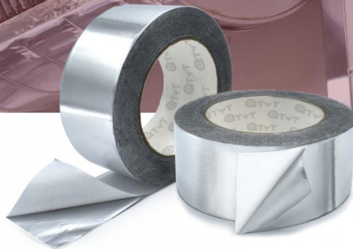
Aluminium tape recovered with an aluminium backing and high performance transparent water-based acrylic adhesive, protected by a 70 g/ m<sup>2</sup> silicone paper liner, which allows easy detachment.
