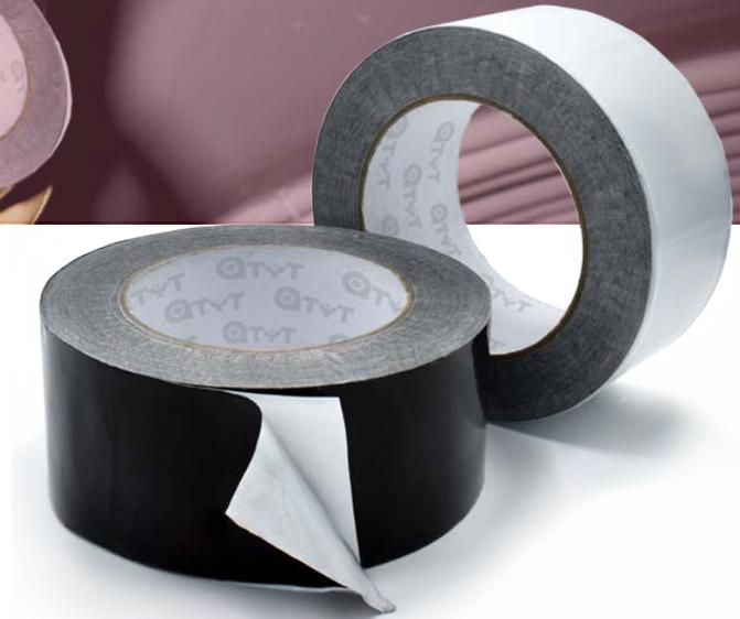
Aluminium tape recovered with an aluminium backing and high performance transparent water-based acrylic adhesive, protected by a 70 g/m<sup>2</sup> silicone paper liner, which allows an easy detachment.
