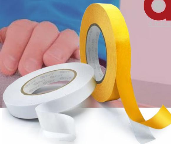
Double-sided tape composed by a non-woven backing tissue coated on both sides with a solvent acrylic adhesive and protected its top-side with a bi-siliconized paper liner.
