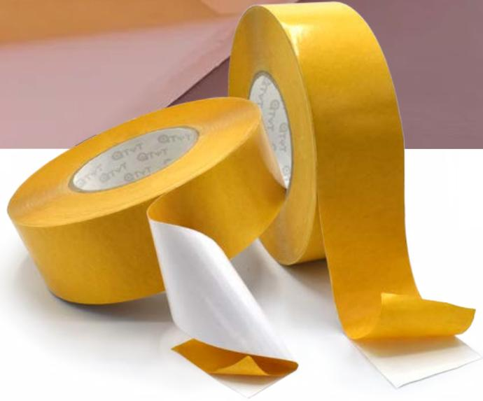
Double-sided adhesive tape composed by an 80 µm PVC backing, covered on both sides by a modified polyacrylic adhesive and protected on its upper side by a 90 g/m<sup>2</sup> yellow bi-siliconized liner.
